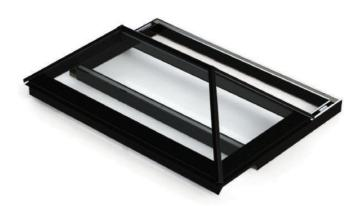
The glazing on your Slide Opening Roof Lantern is angled at 40° on all 4 sides, which will allow the rain to run off. The kerb that you build will therefore need to be level on all 4 sides. As mentioned, the unit always opens across the width and always away from the side that the rain sensor is located.
