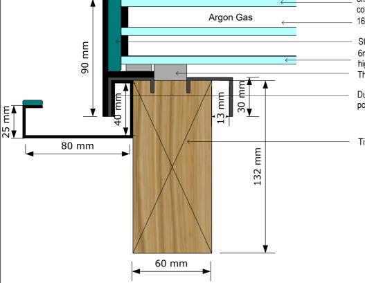
6mm Reflex+ toughened glass solar control easy clean outer panel 16mm Argon gas filled cavity
