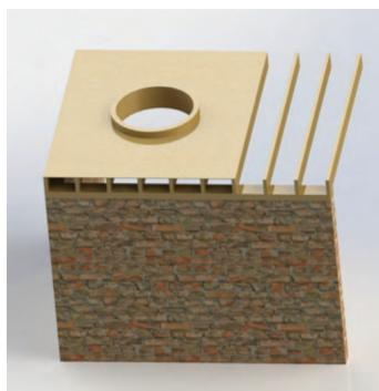
The O-Lite will need to be set at a minimum pitch of 5° (maximum 15°), to prevent water pooling on the surface of the glass.
