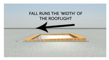
Your Open-Lite Access Rooflight needs a slight pitch of 5°-15° for rain to run off. If your roof does not have this pitch, build the angle into your kerb.
