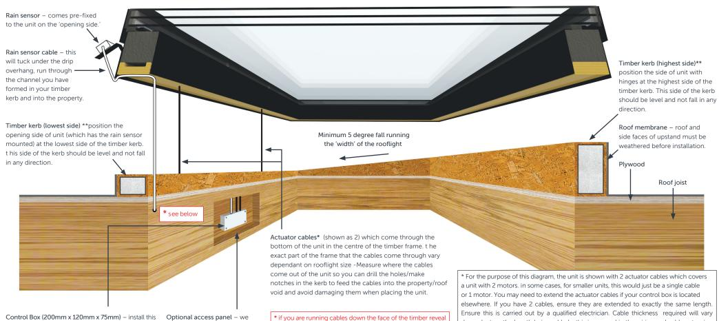
in the void of the roof, between the joists. t his is where your actuator cables and rain sensor cable will be wired in to when you have fed them through into the property. t his is powered by a standard 3 pin plug socket, which you will need to install into this area in advance, positioning within 400mm of the control box location, the control box also acts as the remote receiver.
