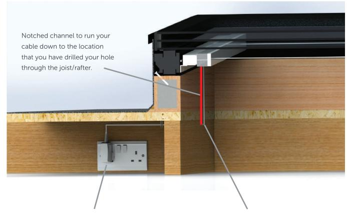
Once you have fed the cable through to the void area in your ceiling, connect it to the 3000mm plug adapter cable provided.
