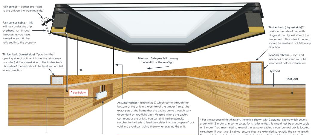
Control Box (200mm x 120mm x 75mm) – install this in the void of the roof, between the joists. t his is where your actuator cables and rain sensor cable will be wired in to when you have fed them through into the property. t his is powered by a standard 3 pin plug socket, which you will need to install into this area in advance, positioning within 400mm of the control box location, the control box also acts as the remote receiver.
