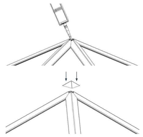
Ensure that the cap goes on neatly and level, wiping away any excess silicone with a damp cloth
