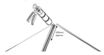
ii) Next run silicone between all the glass panels and frames, on either side of the hip bars, again running approximately 100mm of silicone from each end of the hip bars, top and bottom.
