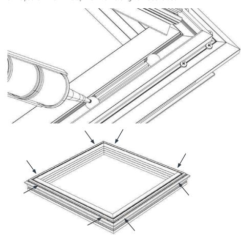
The next stage is to insert the glass sections. The frame is designed so these will fit easily and neatly into place, but care needs to be taken as these are the heaviest components of your roof lantern.
