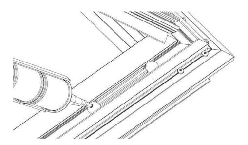
ii) You will require 2 packers per pane of glass (16 total). These will be provided as part of your kit. Position these as per the image below, remembering to put a spot of silicone on either side to prevent them sliding when you position the glass.
