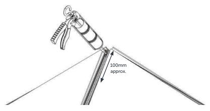
il) Next run silicone between all the glass panels and frames, on either side of the hip bars, again running approximately 100mm of silicone from each end of the hip bars, top and bottom.
