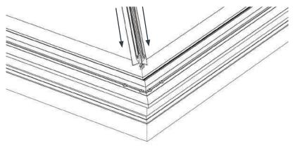
ii) Now pull the hip body toward you whilst tightening the bolt. This will ensure that the internal nut stays in place whilst tightening. Repeat for all 4 corners
