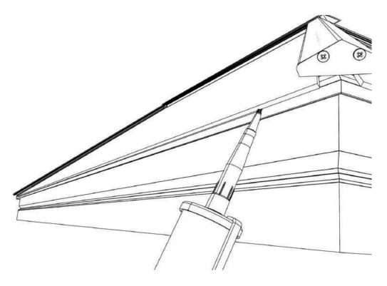
i) From the inside of the lantern, gently remove all of the protective film from the glazing tape on the hip bars.
