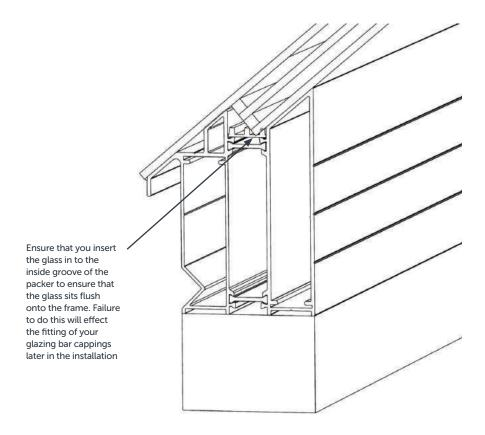
When you are confident that the glass is positioned correctly, you are ready to apply silicone as per the next step.
