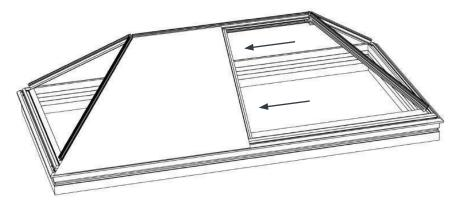
If you also have a split in the triangular end pane of glazing, repeat the same process, ensuring that you use the T-bars with the angled cut at one end. The angled end is to be fitted into the area where the 2 hip bars meet the T-bars.
