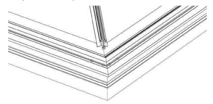
i) The ridge body has blocks located at either end which already house the bolts that will connect to your hip bars. Slide the slotted end of the hip bars over the bolts in the ridge end block. Position the hip bars so they connect with each other in line with the centre of the ridge bar as shown. Tighten the bolts, then repeat at the other end.
