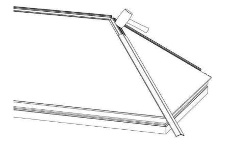
iii) Slide the hip carriers up the hip bar, ensuring that the angled cut-outs line up perfectly and are positioned dead centre to the ridge bar.
