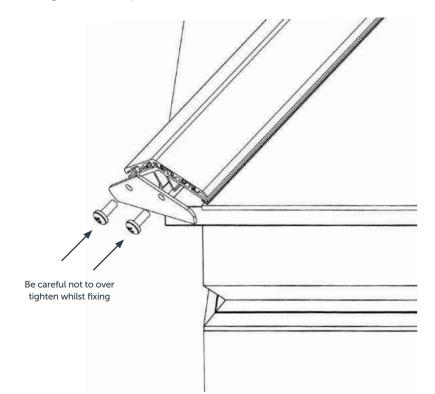
ii) It is now time to fit the two ridge end caps. Fill the space between the end of the ridge cover and the hip caps generously with silicone as shown and apply the two end caps.
