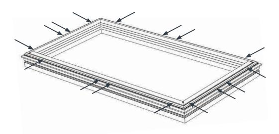
The next stage is to insert the glass sections. The frame is designed so these will fit easily and neatly into place, but care needs to be taken as these are the heaviest components of your roof lantern.
