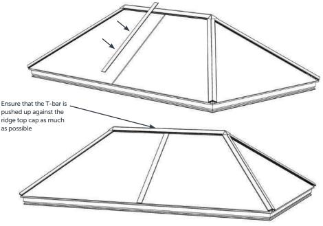
Repeat this on the other side of the lantern. For split triangle end panels (if applicable), ensure that you use the outer T-Bars that have the angled ends and ensure that they are pushed up tight against the hip bars.
