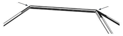
ii) Then slide your ridge top cap in from one end onto the ridge carrier, again, ensuring that it is perfectly centred by checking both ends as shown.
