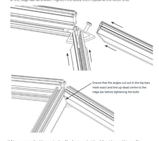
ii) Now pull the hip body toward you whilst tightening the bolt. This will ensure that the internal nut stays in place whilst tightening. Repeat for all 4 corners.
