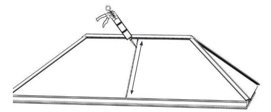
ii) Take one of the longer outer T-bars and remove the entire green protective coverings off the glazing tape, both sides of the central spine. The end of the T-Bar that has the central spine notched out will be positioned at the bottom. Push the T-bar into the silicon to complete the seal, ensuring the top of the T-bar is butted up tightly to the ridge top cap. Press down firmly to ensure the glazing tape sticks to the surface of the glass all the way down.
