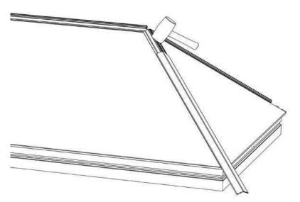
iii) Slide the hip carriers up the hip bar, ensuring that the angled cut-outs line up perfectly and are positioned dead centre to the ridge bar.
