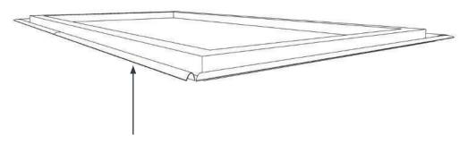
Roof membrane folded back out of the way, leaving the timber upstand exposed for the installation of the roof lantern.
