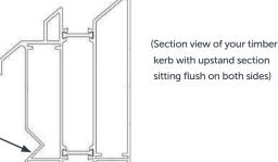
iii) You now need to secure the upstand to the timber kerb by inserting screws into the purpose made groove as shown, about 100mm from each corner, screwing through the upstand into the timber underneath. You will need to predrill your holes into the aluminium frame using a standard metal drill bit.
