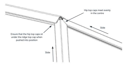
ii) If the plastic hip carrier is protruding from the bottom of the hip bars, use a hacksaw to carefully remove the excess, being careful not to damage the aluminium hip caps. Repeat at each corner if necessary.
