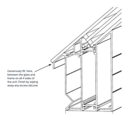
The assembly of your Slimline® lantern is now complete. You are now ready to flash the upstand with your chosen roof membrane.
