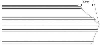
ii) The ends of the ridge carrier might be slightly rough or frayed after doing this, which will effect the ease of sliding your ridge top cap into place during the next step. If this is the case, we advise that you gently shave the ends with a stanley knife, to create a smoother surface
