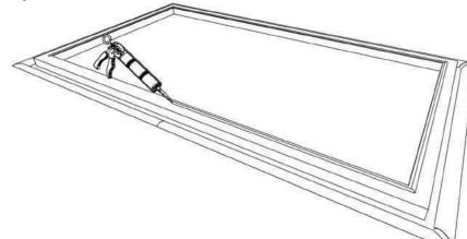
ii) Then carefully place the assembled upstand on to the kerb, ensuring it sits flush with the inner and outer edge of the kerb.
