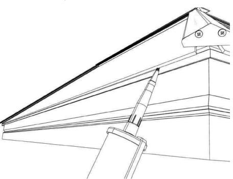
ii) From the inside of the lantern, gently remove all of the protective film from the glazing tape on the hip and ridge bars.
