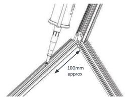
ii) Next run silicone between all the glass panels and frames, on either side of the hip and ridge bars. Only 100mm of silicone is required running from each end of the hip bars. For the ridge bar, run silicone the full length on both sides.
