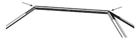
ii) Then slide your ridge top cap in from one end onto the ridge carrier, again, ensuring that it is perfectly centred by checking both ends as shown.
