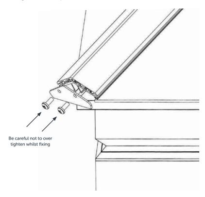
ii) It is now time to fit the two ridge end caps. Fill the space between the end of the ridge cover and the hip caps generously with silicone as shown and apply the two end caps.
