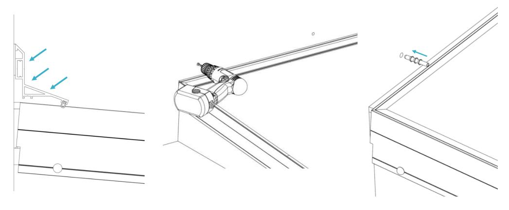
You now need to clean the dust and debris away from the top of the rooflight and foam gasket where it meets the wall, in preparation to seal this area with silicone.
