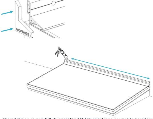
The installation of your Wall abutment Fixed Flat Rooflight is now complete. For internal plaster finishing guidelines, please refer to the roof section diagrams at the end of this guide.
