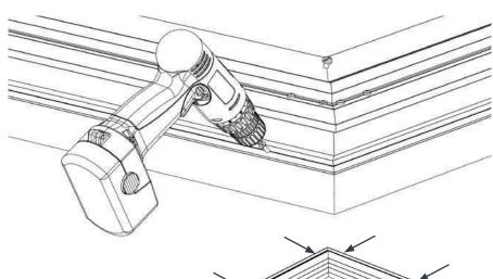
We recommend a minimum of 12 screws - two at each corner, with a further screw in the middle of each side.
