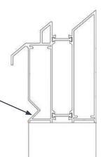
(Section view of your timber kerb with upstand section sitting flush on both sides) iii) You now need to secure the upstand to the timber kerb by inserting screws into the purpose made groove as shown, about 100mm from each corner, screwing through the upstand into the timber underneath. You will need to predrill your holes into the aluminium frame using a standard metal drill bit.
