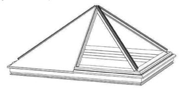
ii) You are now ready to drop in the next panel of glass onto the inside groove of the packers, gently positioning the glass into the frame. Lastly, ensure the T-Bar is positioned exactly in the centre between the 2 panels of glass.
