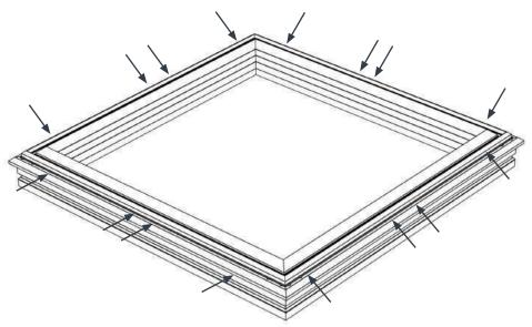
The next stage is to insert the glass sections. The frame is designed so these will fit easily and neatly into place, but care needs to be taken as these are the heaviest components of your roof lantern.
