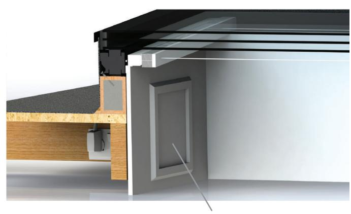
When you have plastered your reveals leading up to the rooflight, you have the option of installing an access panel in this area.
