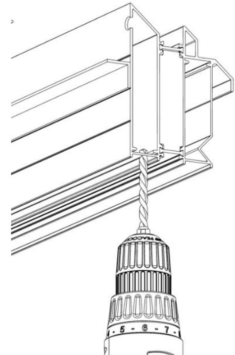
**You will be drilling into the first chamber again, as shown, vertically in line with the first hole you drilled.**
