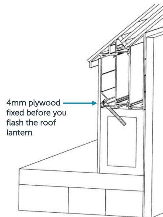
**Your roof lantern assembly is now complete.** For internal plaster finishing details please refer to the roof cross section fitting guide, located on page 8 of this guide. Following this, you will find the wiring guides for electronic vents.
