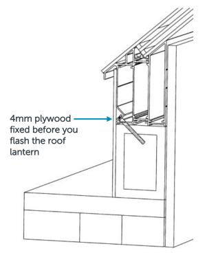
Your roof lantern assembly is now complete. For internal plaster finishing details please refer to the roof cross section fitting guide, located on page 8 of this guide. Following this, you will find the wiring guides for electronic vents.
