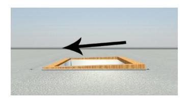
Your Fixed Flat Rooflight needs to be pitched at a minimum of 5° to allow water run-off. If your roof does not have this pitch, build the angle into your timber kerb. We recommend that you run the fall across the 'width' or 'shorter side' of the rooflight when building an angled kerb, as the fall will be less noticeable, which will improve the aesthetics when fitted.
