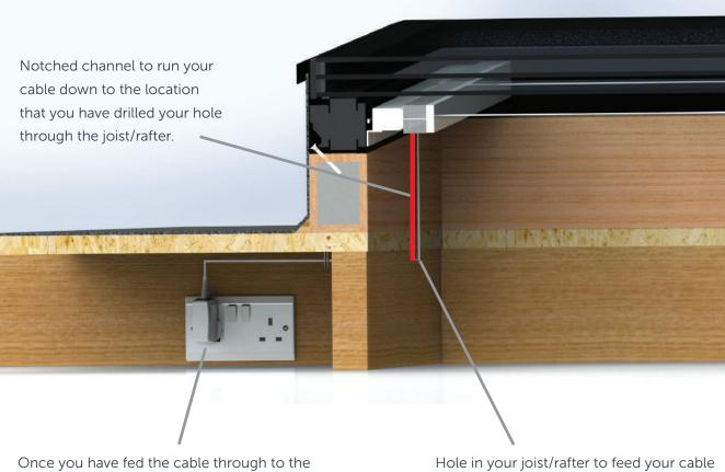
Once you have fed the cable through to the void area in your ceiling, connect it to the 3000mm plug adapter cable provided.
