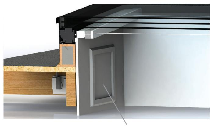
When you have plastered your reveals leading up to the rooflight, you have the option of installing an access panel in this area.
