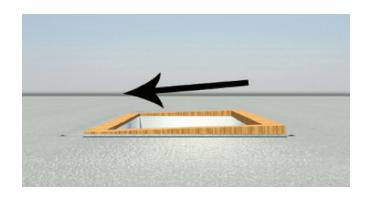
Your Fixed Flat Rooflight needs to be pitched at a minimum of 5° to allow water run-off. If your roof does not have this pitch, build the angle into your timber kerb. We recommend that you run the fall across the 'width' or 'shorter side' of the rooflight when building an angled kerb, as the fall will be less noticeable, which will improve the aesthetics when fitted.
