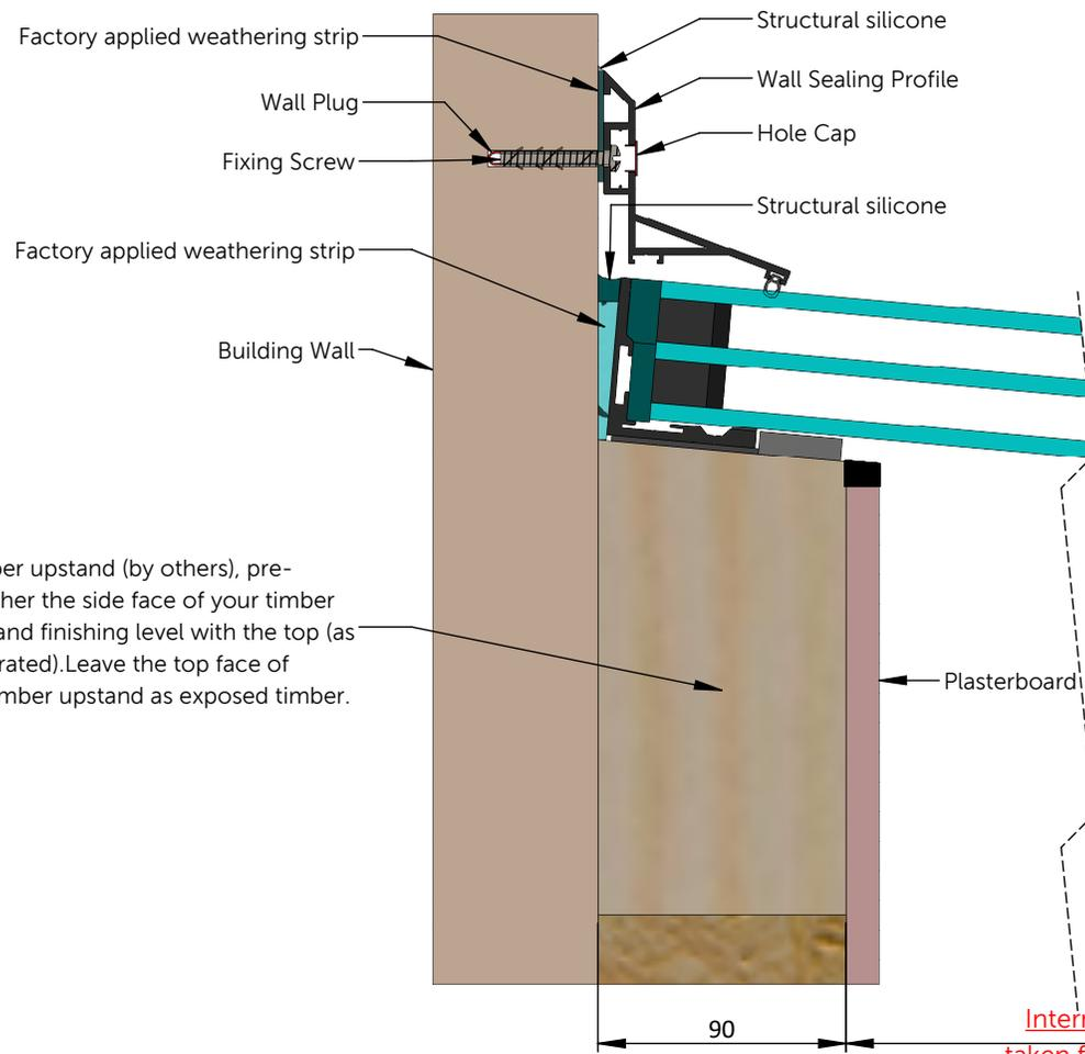
Timber upstand (by others), pre-weather the side face of your timber upstand finishing level with the top (as illustrated). Leave the top face of the timber upstand as exposed timber.
