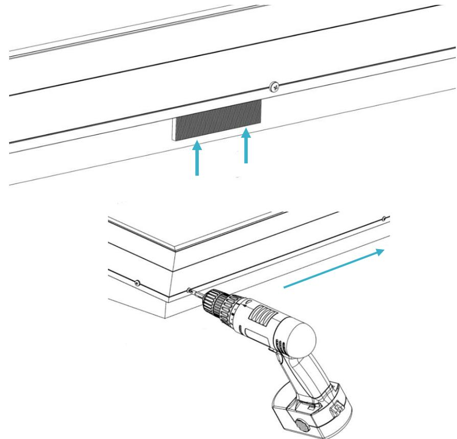
You can now use the provided screw caps to conceal the screws that you have inserted into the front and two sides of the rooflight.
