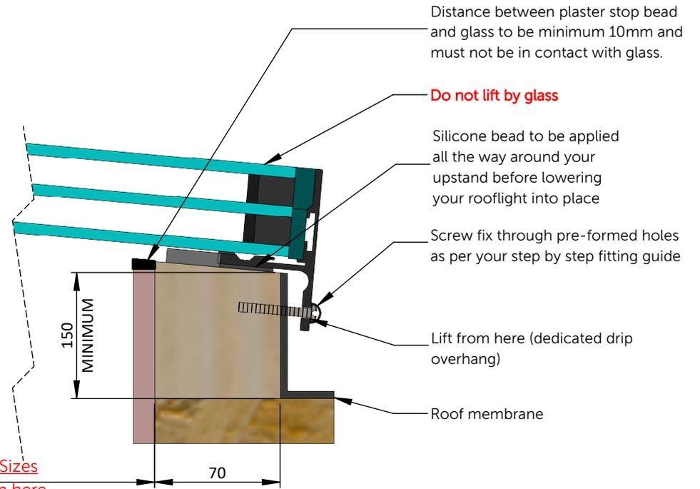
Internal Sizes taken from here (size ordered = size of timber structural opening)
