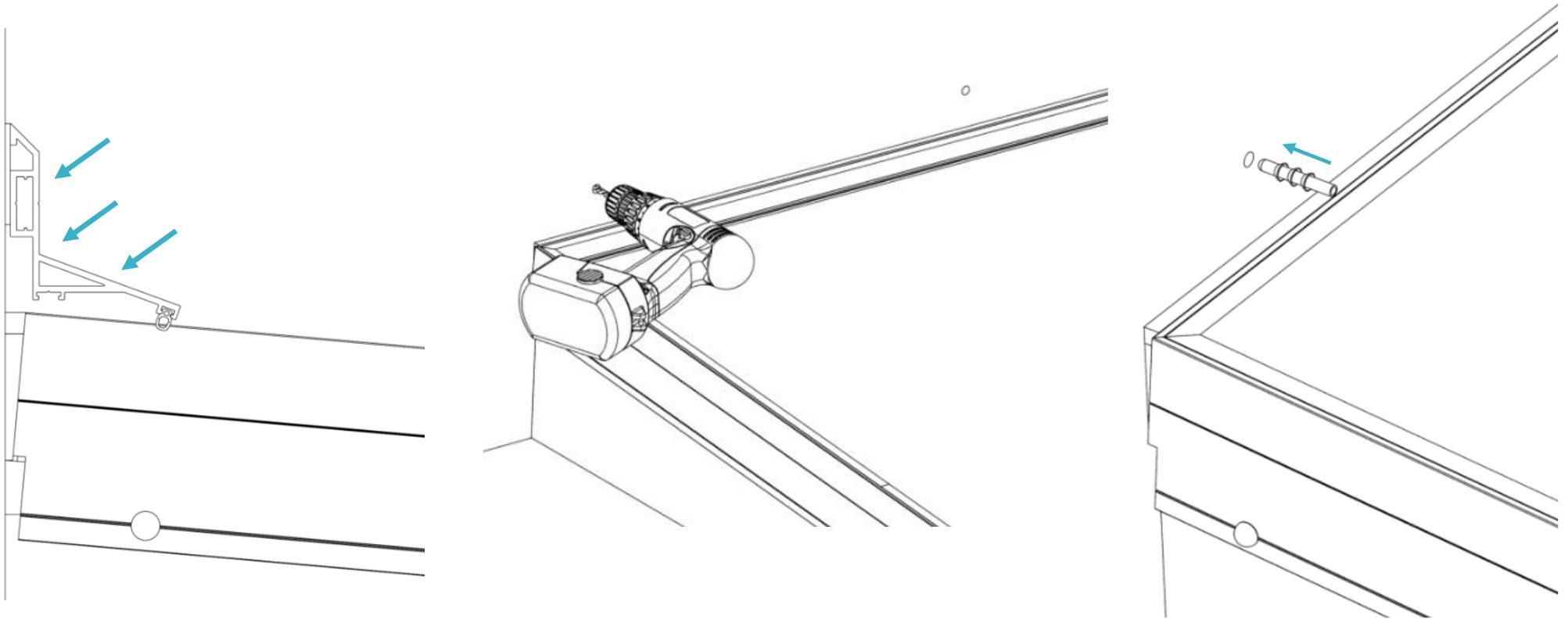
You now need to clean the dust and debris away from the top of the rooflight and foam gasket where it meets the wall, in preparation to seal this area with silicone.
