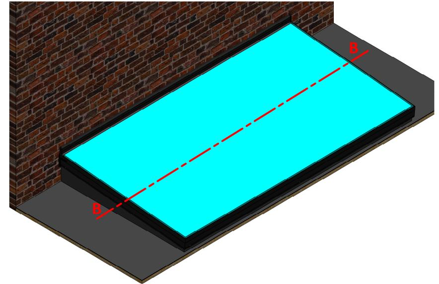
Distance between plaster stop bead and glass to be minimum 10mm and must not be in contact with glass.
