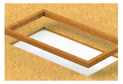
You will need to incorporate a 1<sup>0</sup> fall into your timber kerb, to allow for water runoff. We recommend you run the finished floor level, at the same angle so it sits flush with the top pane of glass. Bear this in mind when creating your timber kerb, also taking the depth of the unit into account, as mentioned in the introduction.
