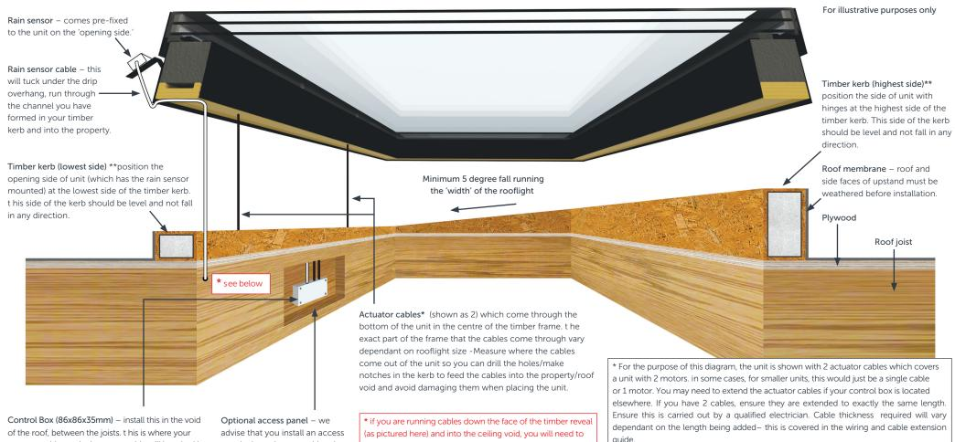
actuator cables and rain sensor cable will be wired in to when you have fed them through into the property. t his is powered by a standard 3 pin plug socket, which you will need to install into this area in advance, positioning within 400mm of the control box location, the control box also acts as the remote receiver.
