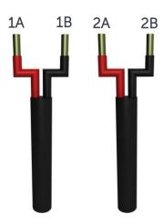
Slide opening flat rooflights and lanterns will always have 2 actuator cables. Wire in to the output pairs, as per the above diagram
