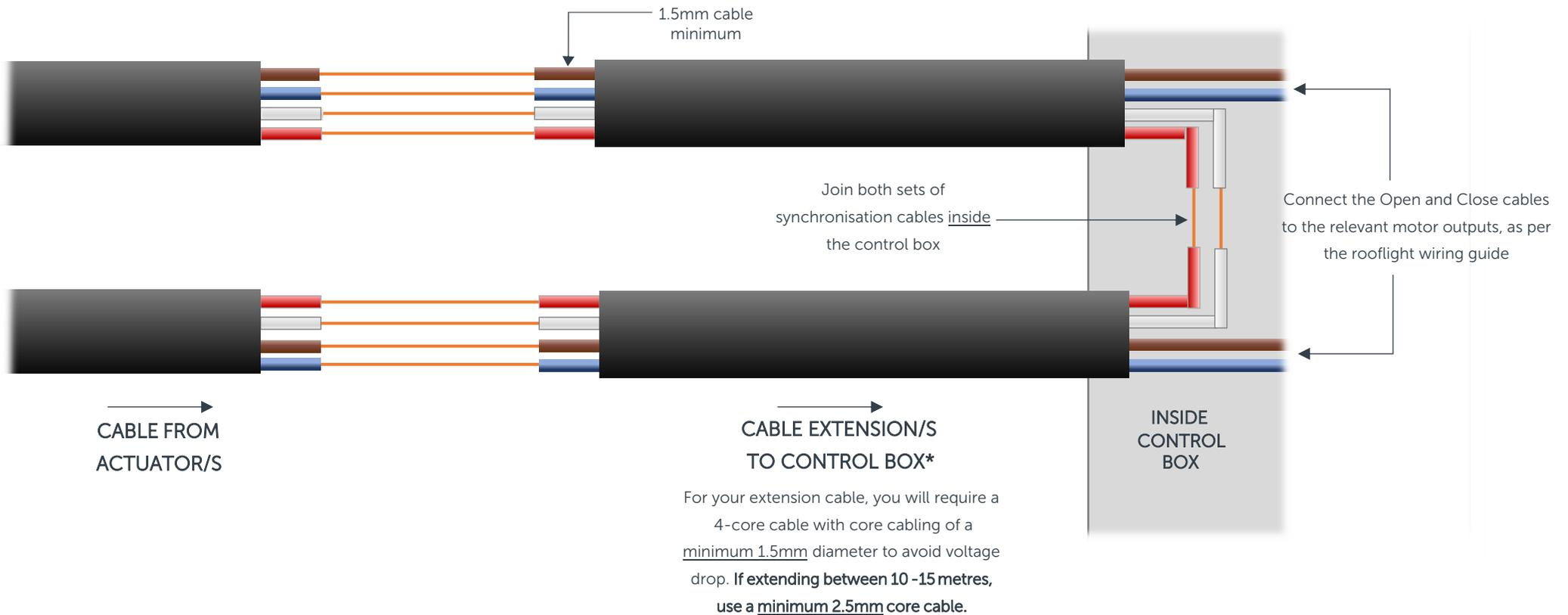
*\*If your rooflight has 2 actuator cables that need to be extended, please ensure they are extended to exactly the same length to avoid the motors operating at different speeds.*
