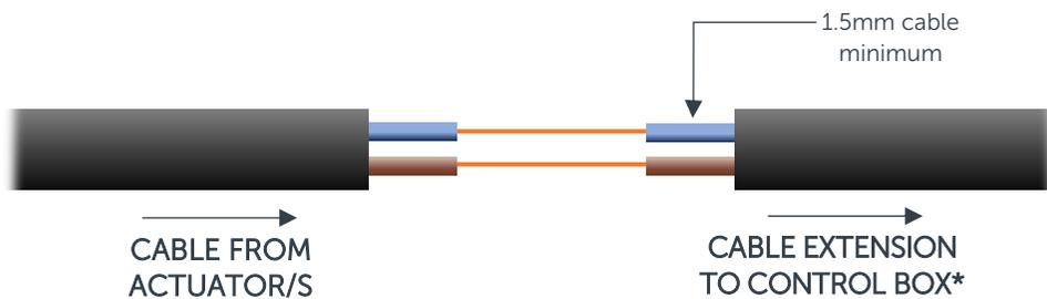
For your extension cable, you will require a 2-core cable (minimum) with core cabling of a minimum 1.5mm diameter to avoid voltage drop, up to 10 metres. **If extending between 10-15 metres, use a minimum 2.5mm core cable.**
