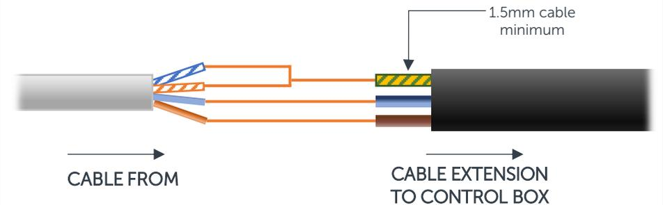
Rain sensor cable will be a 4-core cable;
