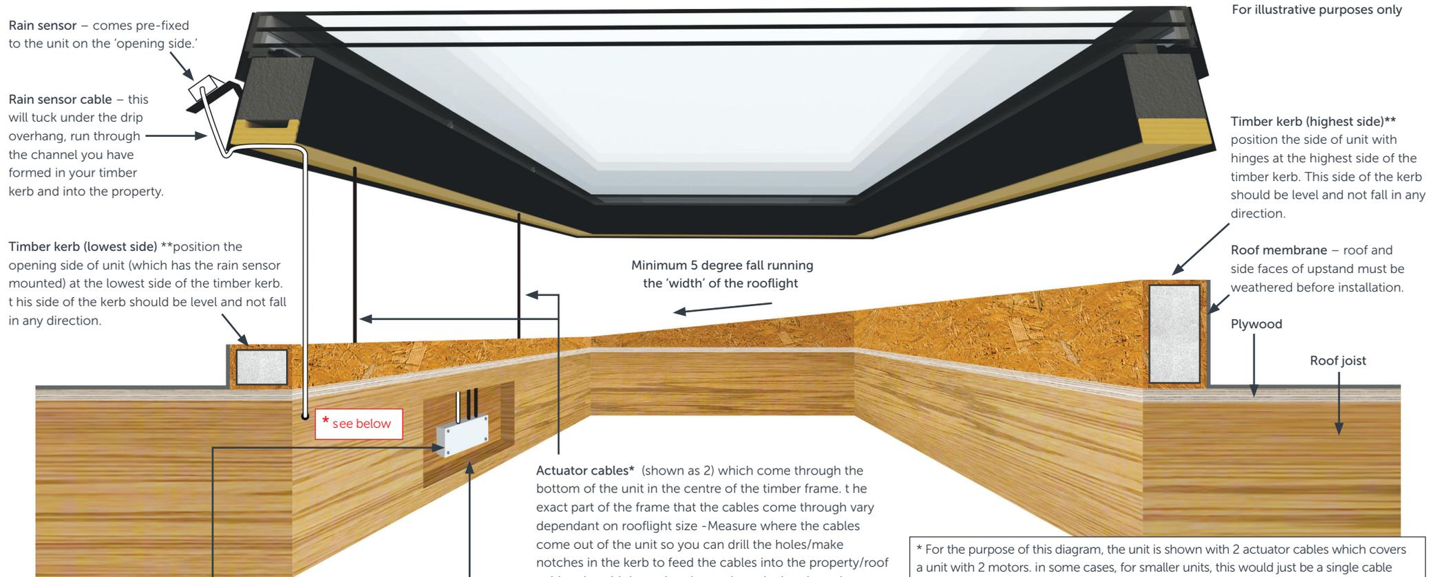
**Control Box (86x86x35mm)** – install this in the void of the roof, between the joists. This is where your actuator cables and rain sensor cable will be wired in to when you have fed them through into the property. This is powered by a standard 3 pin plug socket, which you will need to install into this area in advance, positioning within 400mm of the control box location. The control box also acts as the remote receiver.
