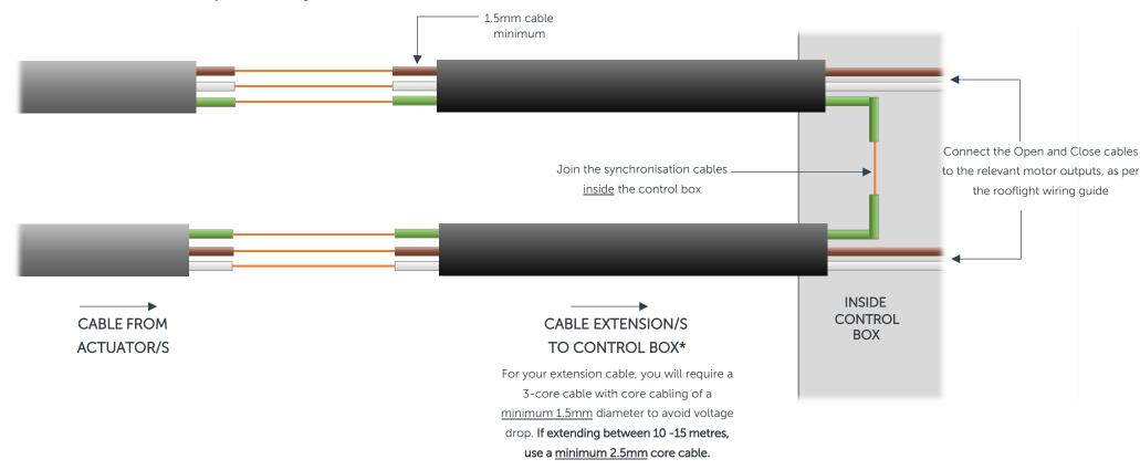
\*If your rooflight has 2 actuator cables that need to be extended, please ensure they are extended to exactly the same length to avoid the motors operating at different speeds.
