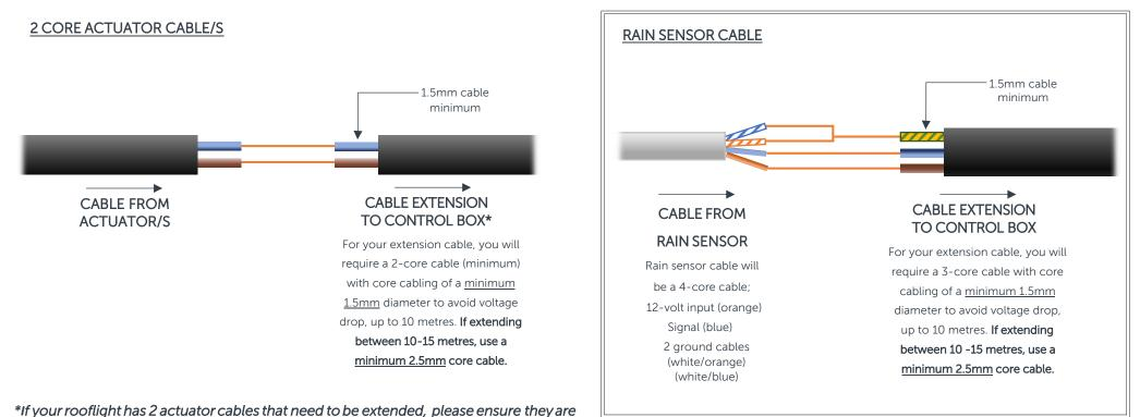
extended to exactly the same length to avoid the motors operating at different speeds.
