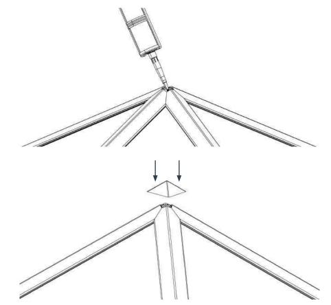
Ensure that the cap goes on neatly and level, wiping away any excess silicone with a damp cloth
