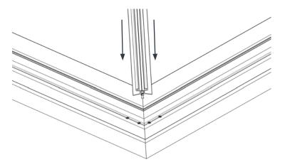
ii) Now pull the hip body toward you whilst tightening the bolt. This will ensure that the internal nut stays in place whilst tightening. Repeat for all 4 corners
