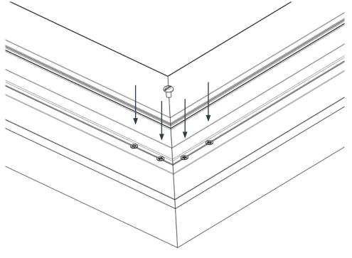
iv) Turn the upstand over and repeat the same process for each corner on the underside of the unit. Fixing the screws through each pre-formed hole. Once complete, the frame should be securely fastened together.
