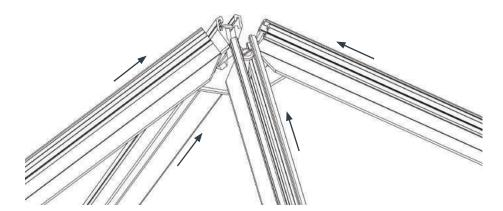
Ensure that the angled cut outs on your hip bars line \_\_\_\_ up perfectly on all 4 sides as shown here. You can then tighten all 4 bolts to brace the 4 bars together
