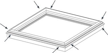
The next stage is to insert the glass sections. The frame is designed so these will fit easily and neatly into place, but care needs to be taken as these are the heaviest components of your roof lantern.
