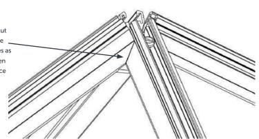
ii) Now remove the blue protective film from each side of the ridge and hip profiles.
