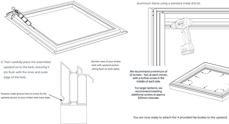
iii) You now need to secure the upstand to the timber kerb by inserting screws into the purpose made groove as shown, about 100mm from each corner, screwing through the upstand into the timber underneath. You will need to predrill your holes into the aluminium frame using a standard metal drill bit.
