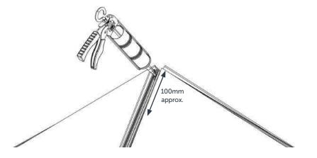
il) Next run silicone between all the glass panels and frames, on either side of the hip bars, again running approximately 100mm of silicone from each end of the hip bars, top and bottom.
