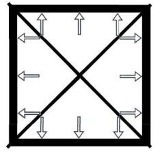
We recommend a minimum of 12 screws - two at each corner, with a further screw in the middle of each side.
