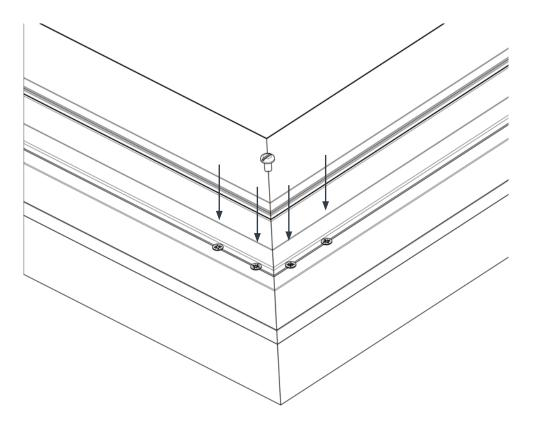
iv) Turn the upstand over and repeat the same process for each corner on the underside of the unit. Fixing the screws through each pre-formed hole. Once complete, the frame should be securely fastened together.
