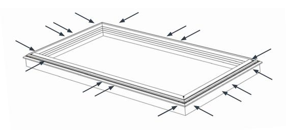
The next stage is to insert the glass sections. The frame is designed so these will fit easily and neatly into place, but care needs to be taken as these are the heaviest components of your roof lantern.
