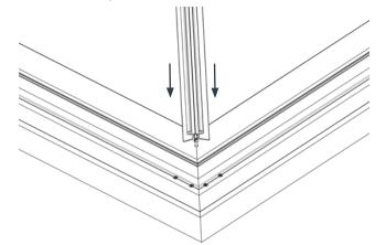
ii) Now pull the hip body toward you whilst tightening the bolt. This will ensure that the internal nut stays in place whilst tightening. Repeat for all 4 corners.
