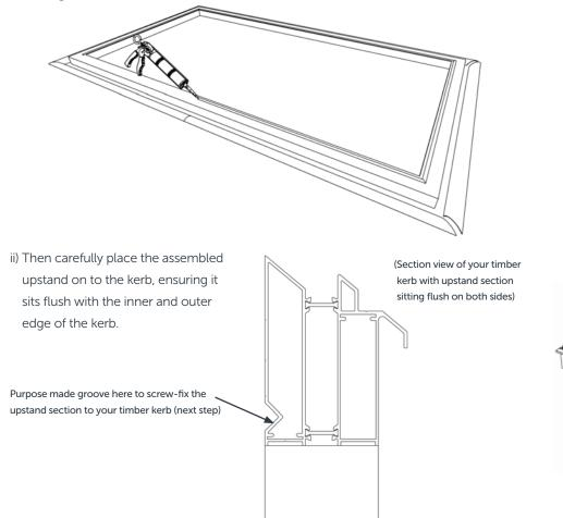
iii) You now need to secure the upstand to the timber kerb by inserting screws into the purpose made groove as shown, about 100mm from each corner, screwing through the upstand into the timber underneath. You will need to predrill your holes into the aluminium frame using a standard metal drill bit.
