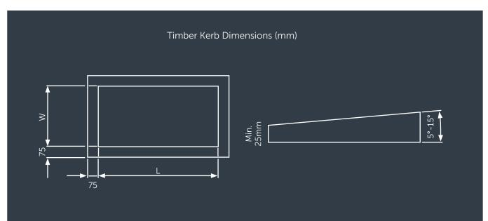
Dimensions L and W are the length and width of your Fixed Flat Rooflight respectively. The internal dimensions are equal to the size ordered.
