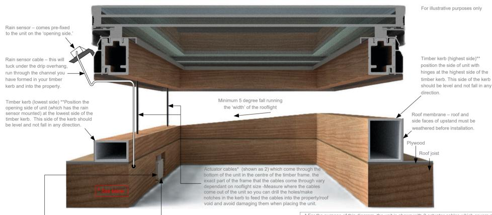
Control Box (86x86x35mm) – install this in the void of the roof, between the joists. t his is where your actuator cables and rain sensor cable will be wired in to when you have fed them through into the property. t his is powered by a standard 3 pin plug socket, which you will need to install into this area in advance, positioning within 400mm of the control box location. t he control box also acts as the remote receiver.
