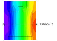
This product featureThis product features a Wood Plastic Composite (WPC) profile as a 60mm wide thermal break which is filled with phenolic foam core to give a composite U-Value of 0.365 W/(m2K) WPC advantages over wood are clear sustainable credentials using recycled wood chip and plastic waste to produce a super insulating material that has good shape retention in high temperatures thanks to the inclusion of ceramic material within the material formula.
