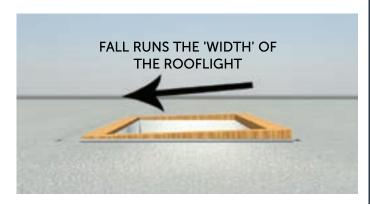
Your hinged opening rooflight needs to be pitched between 5°-15° for rain to run off. If your roof does not have this pitch, build the angle into your kerb.
