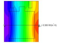
This product featureThis product features a Wood Plastic Composite (WPC) profile as a 60mm wide thermal break which is filled with phenolic foam core to give a composite U-Value of 0.365 W/(m2K) WPC advantages over wood are clear sustainable credentials using recycled wood chip and plastic waste to produce a super insulating material that has good shape retention in high temperatures thanks to the inclusion of ceramic material within the material formula.
