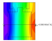
This product featureThis product features a Wood Plastic Composite (WPC) profile as a 60mm wide thermal break which is filled with phenolic foam core to give a composite U-Value of 0.365 W/(m2K) WPC advantages over wood are clear sustainable credentials using recycled wood chip and plastic waste to produce a super insulating material that has good shape retention in high temperatures thanks to the inclusion of ceramic material within the material formula.
